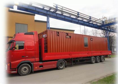
BRODOGRADILIŠTE V. LENAC Steam container boiler room 3000 kg/hr steam 12,6 bar
