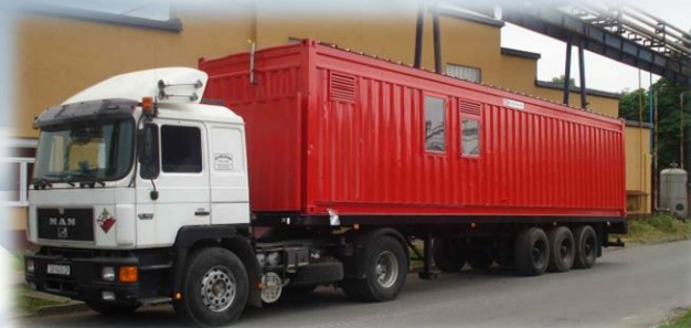
AFROTROPIC COCOA PROCESING Co. Ltd., Gana Steam container boiler room, 600 kg /hr - 12,6 bar
