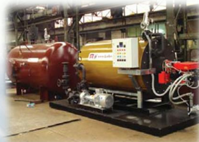
LUKA BAR, VKS 700 Thermal oil heater 1 x 700 kW
